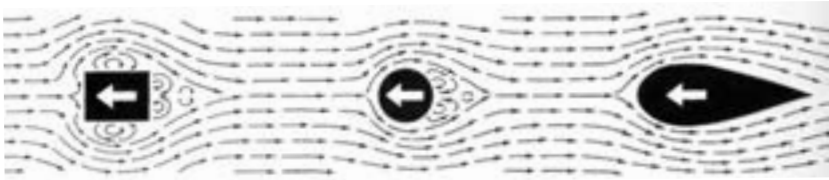
Diagram Illustrating the principle of streamlining , Tiré du livre Horizons de Norman Bel Gedes.
